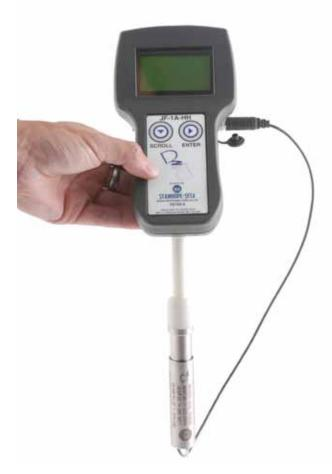
**Conductivity Measurement of Oils**
