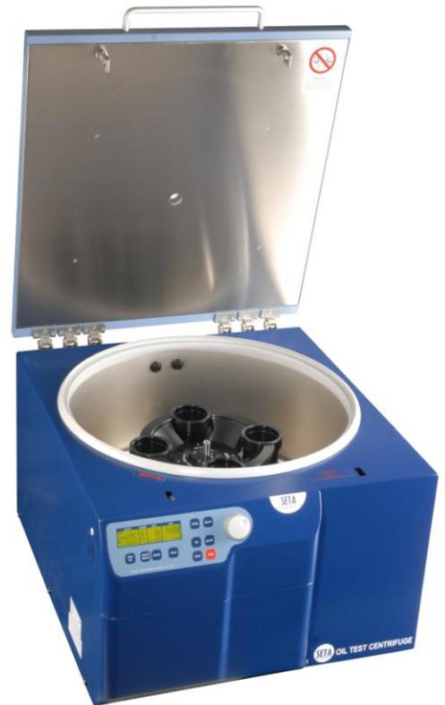
The Seta Oil Test Centrifuge is a microprocessor controlled, heated centrifuge which is specifically designed to meet oil test parameters for determining sediment and water in crude oil.
