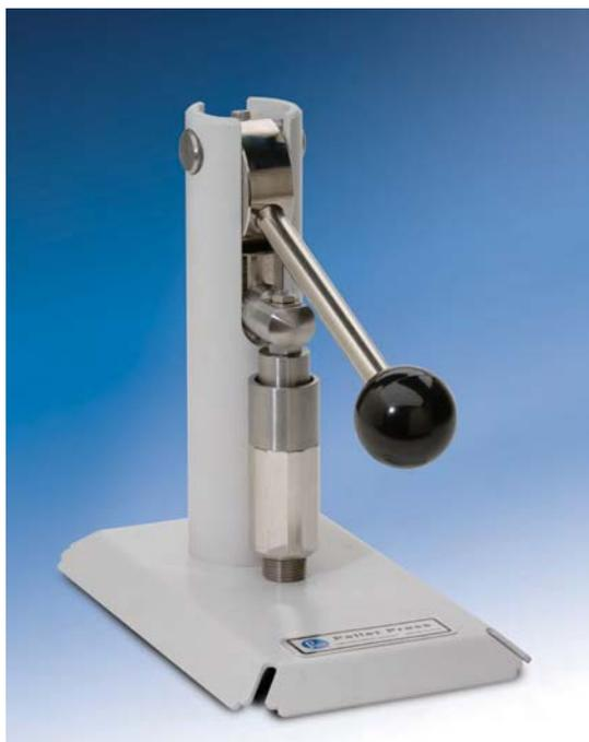
The Parr 2811 Pellet Press provides a convenient means for compressing powdered materials into pellet or tablet form without a heavy investment in expensive tablet-making machinery. It is a compact, hand-operated press that can be used anywhere in the laboratory, requiring very little bench space and no fixed mounting, producing uniform pellets in a polished stainless steel die and ejecting them smoothly into a stainless receiver without danger of contamination.
