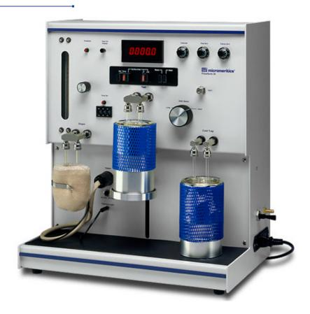
The Flowsorb III 2305 / 2310 provides single-point and multipoint BET surface area measurements with speed, accuracy, and reliability. Samples having surface areas from 0.01 m²/g to over 1,000 m²/g are easily accommodated.
