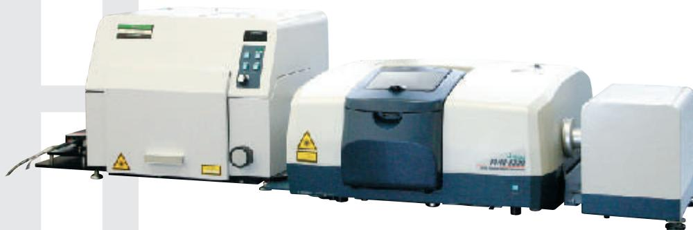
The JASCO Model RFT-6000 FT-Raman accessory is designed for quick, non-destructive FT-Raman analysis of virtually any sample when used in conjunction with the JASCO Model FT/IR-6300 spectrometer.
