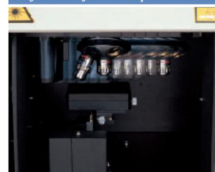
The condensing lens section integrated into the linear slide bench, and micro/macro switching is easy. Mapping measurements can also be supported by using an autostage. And by using the optional TV monitor system (standard with the micro-system), it is possible to verify the measurement site.
