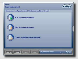
Start the measurement. After the start of the measurement the user is guided through the measuring sequence. Detecting the surface, immersing the measuring body and the measurement itself are all carried out fully automatically. The averaged result, the raw data and all measuring parameters are clearly shown.
