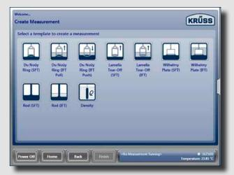
Select measuring method. Measuring templates with standard parameters are included; these are suitable for most cases.
