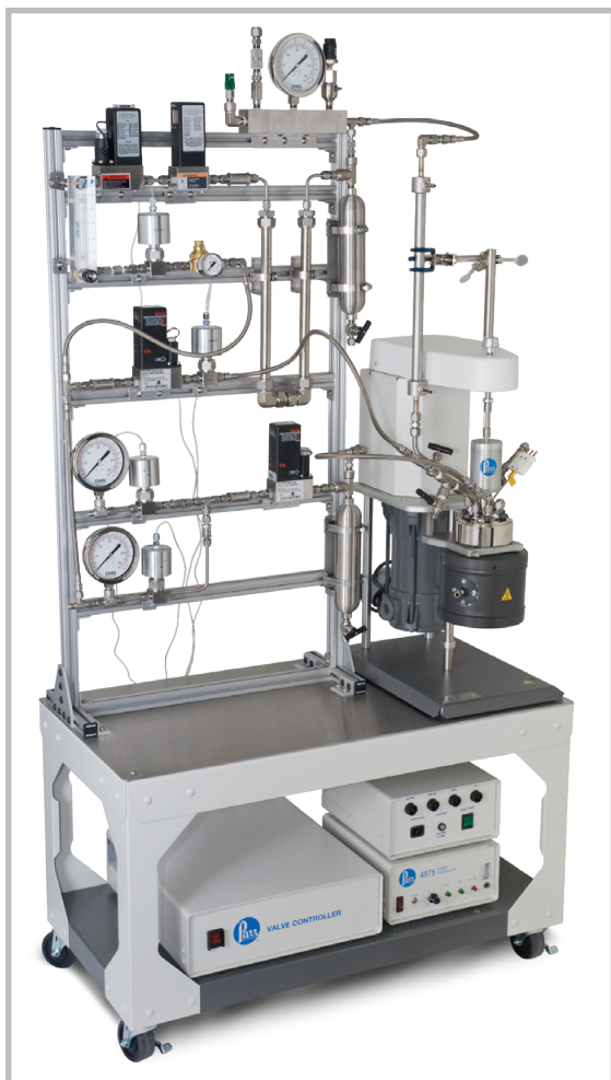
This continuous flow stirred reactor system is on a cart with our Modular Frame System. This modular frame allows for easy access and flexibility in hook-ups, accessories, and flow, including an interchangeable tubular reactor.
